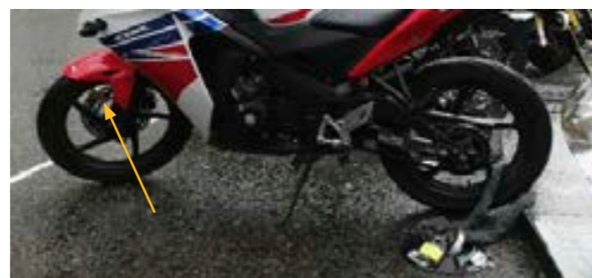
Figure 1 – A motorcycle with a chain and lock securing the rear wheel to a ground anchor. Ideally the lock needs to be elevated or wrapped around the wheel to prevent it being smashed against the ground with a hammer. A yellow disc lock (highlighted by the arrow) secures the front wheel.
