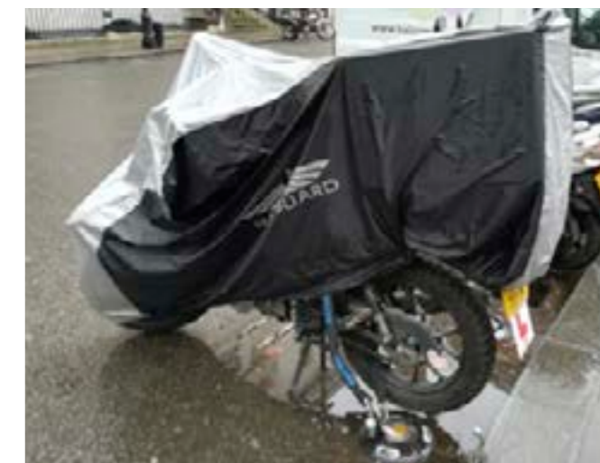
Figure 4 – A lock and chain set has been attached to a ground anchor, but the chain has also been run through the rear wheel and frame. A bike cover also adds a further layer of security to delay or deter a thief, not just waterproofing.
